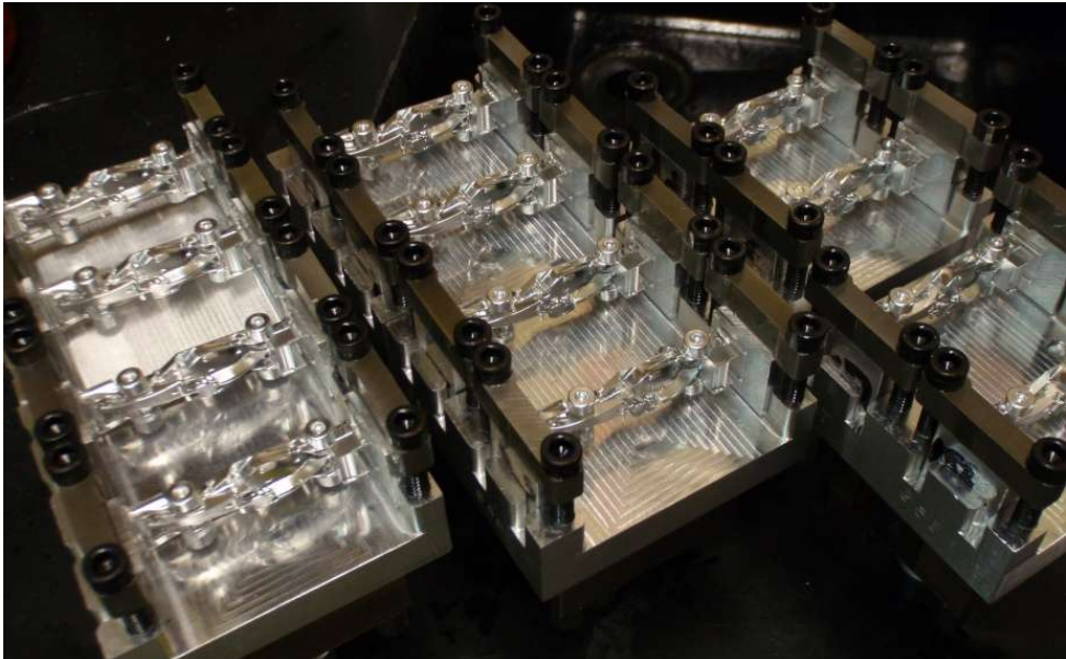
Figure 3: 1st Generation Custom Manually Indexing Fixtures In Use
